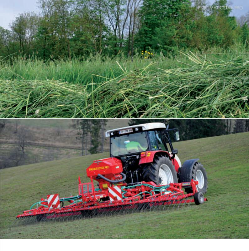
**Six support wheels** guide the frame also in high working speed smoothly, without shaking and with exact depth guidance across the grassland.
