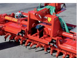
The **rotor tines** - specially designed for grassland and work without problems even in stony soils – ensure that not too many stones are brought up to the surface. The line spacing is 50 mm, which ensures working the full surface in just a 3 cm working depth.
