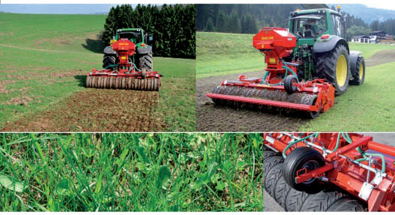
The **seeding roller is driven** by an air wheel which is pressed on the farmflex roller. The seeds are spread in between the rotor (protected by a cover) and the roller.
