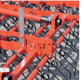
The aggresiveness of the spring tines can be adjusted via a **central lever** per each section in 5 different positions. When folding to the transport position the tines should be adjusted to the flattest position.
