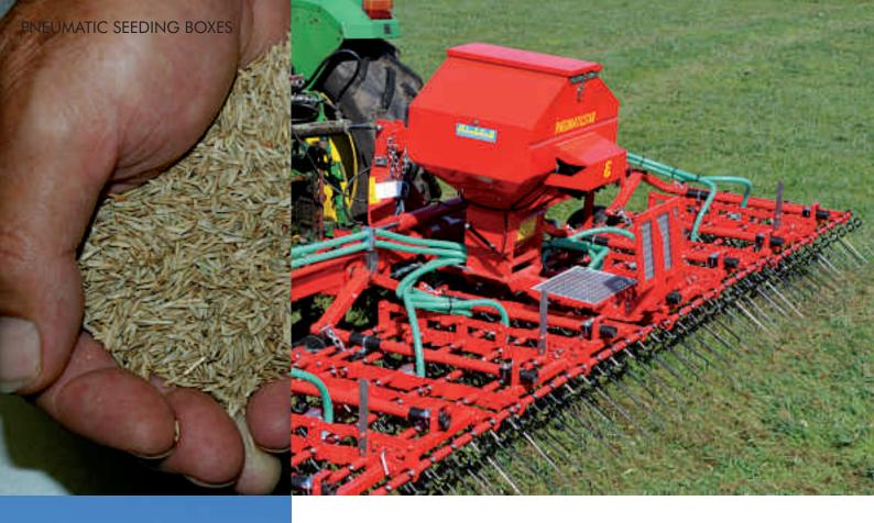
With the **mechanical fan** you can, due to the higher airstream, distribute heavier seeds up to 6 m working width and you can work with increased working speed. Recommended for communities and contractors.
