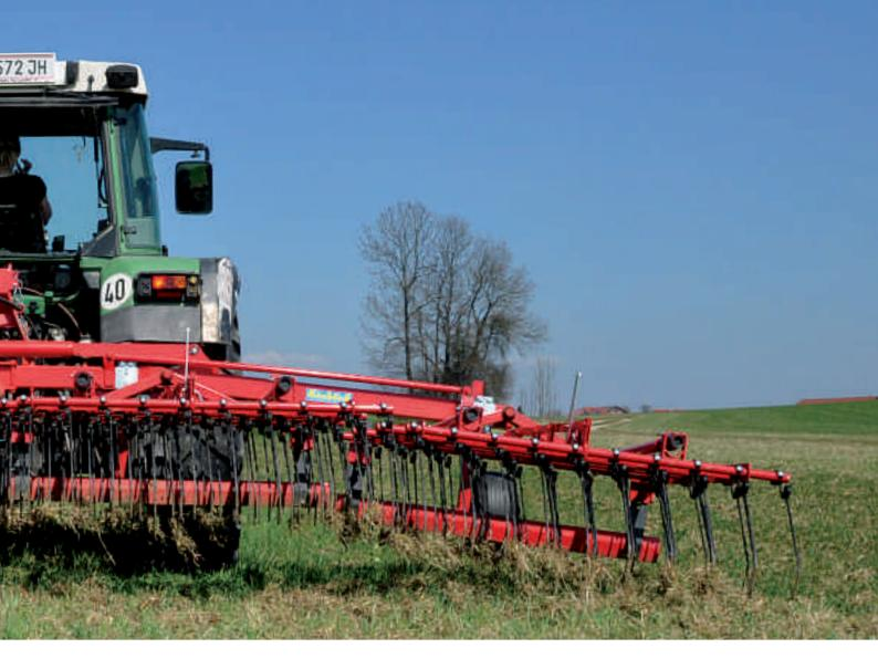
By taking away or mounting of the stop bar on the wing (only on machines without shear retraction) the machine **follows the contours of the land surface** perfectly. The **transportation lock** is unlocked via a rope pull (only on machines without shear retraction).
