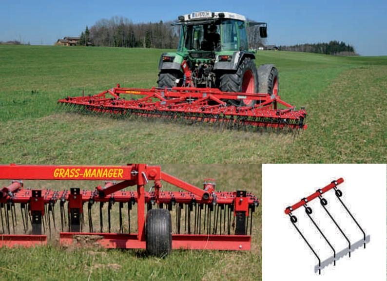
In front of the weeder section a levelling plate can be mounted, which is overload-protected by a leaf spring. This **levelling plate** is height adjustable and ensures an excellent **distribution and levelling of molehills**. In addition, it distributes and levels manure and slurry. It can easily be retro-fitted. For small molehills which appear in a small number, **grassland sheets** which are bolted directly onto the tines can be used.
