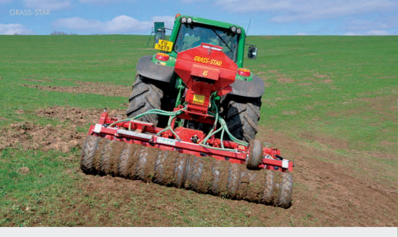
The Farmflex rubber roller, depth adjustable via a breadboard and with ø 520 mm, ensures an **optimal reconsolidation**.
