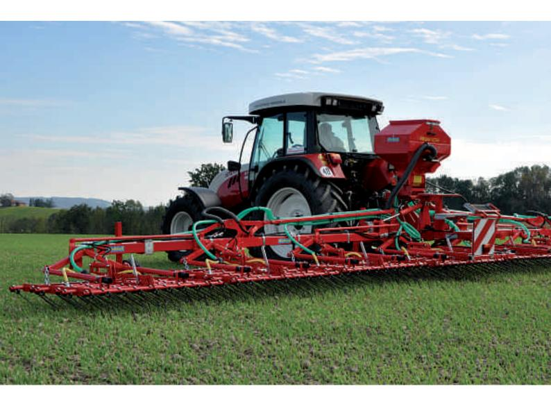
The PNEUMATICSTAR is also suitable for underseeding. **Seeding of clover or clover/grass into grain can collect up to 100 kg nitrogen/ha.** Fields with cover crops are very environmentally friendly due to the good nitrogen balance. Underseeding of grass in maize provides the following advantages:
